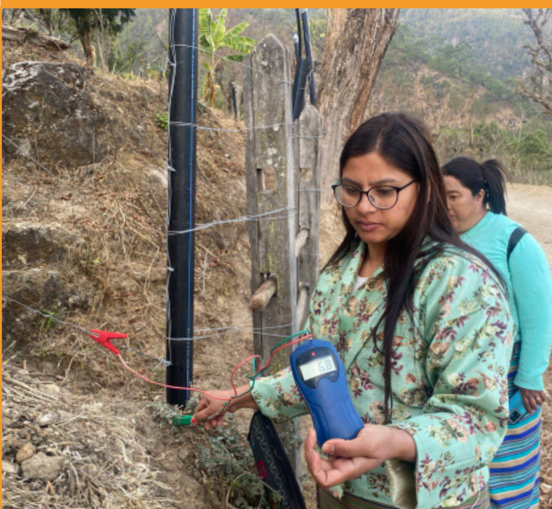
Installation and testing of electric fencing by Agricultural Extension Officer and Local Government team in Kewana Tshachuphu Chiwog, Punakha District
