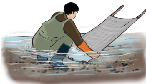
2. Position the net at 45° angle with button fixed at the substrate
