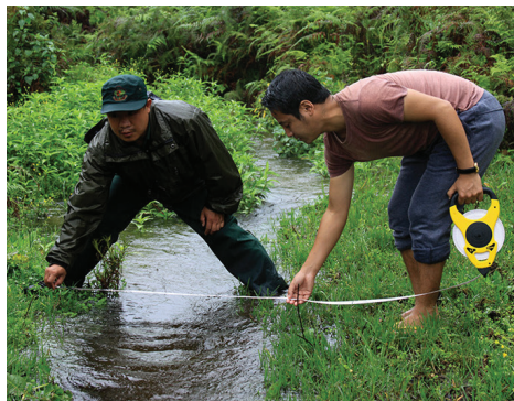
Assessment team measuring the length of a stream to measure velocity and volume by float method.
